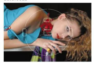
The FinePix S2 Pro incorporates five area AF sensors covering a wide area along both the horizontal and the vertical axes. This generous autofocus coverage is ideal for fast, creative composition. Alternatively the photographer can designate any of the five sensors as primary sensor, allowing highly effective action and sequence photography.
